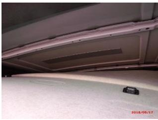
22 Peeling back the rubber around the windows, the liner pulls down to check the clear area for the hole.
