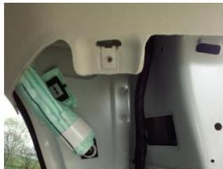
5 fit up under the roof liner. Green stuff is the air bag so be careful not to damage.
