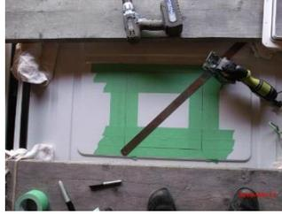
26 Front and back lines are drawn on the tape and diagonals checked for square.
