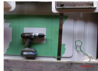
24 By drilling a hole through the roof and liner half way back on the panel
