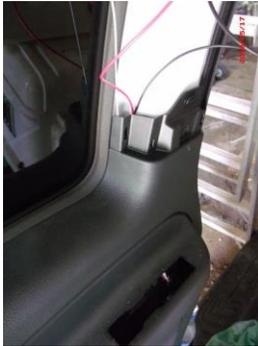
37 and then down to the floor and forward to the fuse block on the auxiliary battery. The cup holder pulls out for access.
