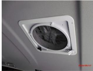
38 Four screws hold the surround in place. Because the infra-red remote sensor is somewhat hidden from the front seat,
