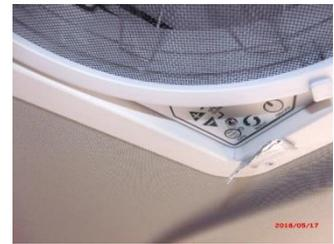
39 A small piece of foil is positioned to reflect the beam up.
